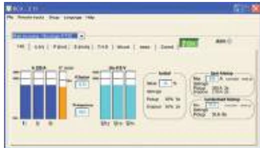
PC screen with motor thermal image and value monitoring.
